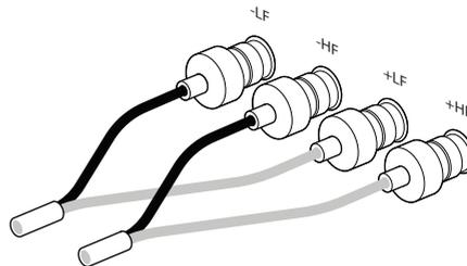
Ask your dealer for advice when selecting speaker cable. Keep its total impedance below the maximum recommended in the speaker specification and use a low inductance cable to avoid attenuation of high frequencies.
